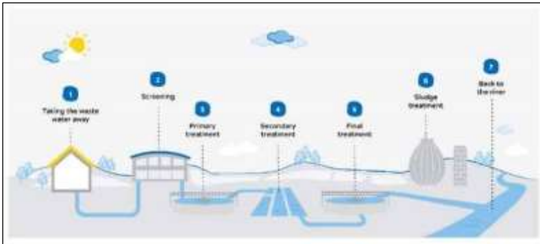
Figure 2.2: Treatment process overview
